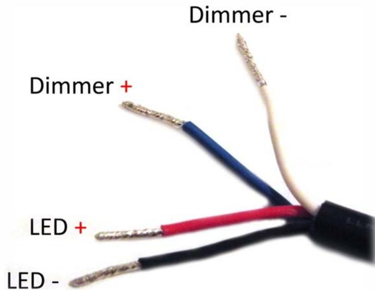
There are 4 output wires on a dimmable driver as in the above photo. The dimming wires, DIM + (blue), and DIM – (white), simply hook up to the respective ports on your controller or dimmer. Dimmable drivers must have the dimmer wires hooked up to a controller or dimmer or the LEDs will not light up. No dimming signal = 0% brightness.
