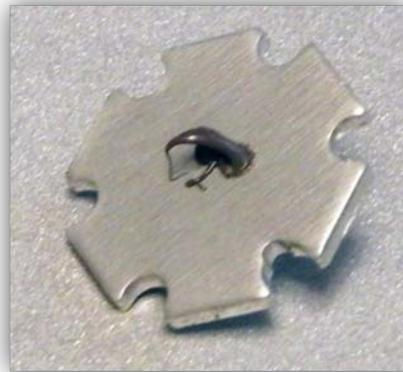
Here's an example of some nicely attached LEDs on one of our Nano Retrofit heatsinks:
